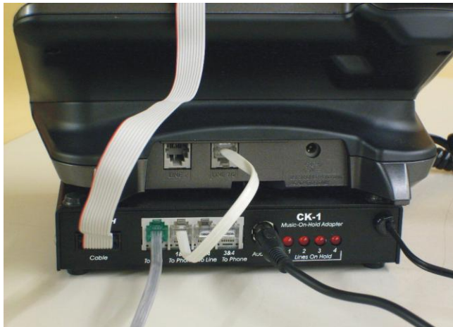
PANASONIC KXTG9392T with skutch CK-1P6 installed. The cables provide (from left to right) connection between sensor board and CK-1P box; dial tone from phone jack; dial tone from CK-1P6 box to PANASONIC phone; audio from on hold music player to CK-1P6.
