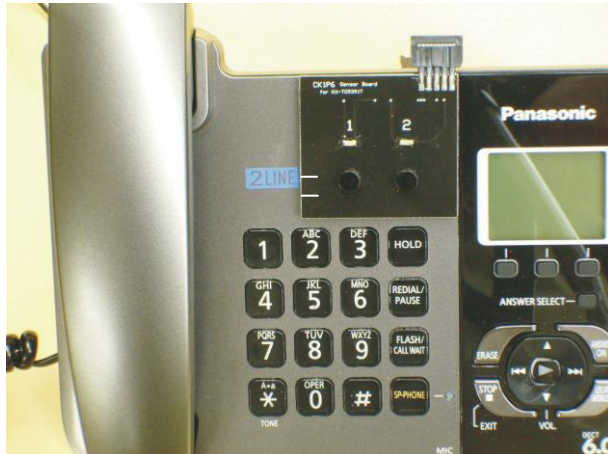
PANASONIC KXTG9392T with SKUTCH CK-1P6 sensor board installed. Note alignment is made easy using the top and right edges of the phone keypad area and alignment guide on the left, near the phone's graphic "2-LINE".
